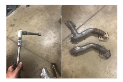
11. When reinstalling the up pipe it is recommended to apply high temp anti size to the threads to not only help with installation but also ease removal in the future. Slide the new up pipe into place with the new gaskets in place and tighten to 28ftlbs.
