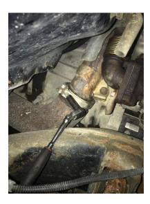
2. Remove the bolt holding the down pipe to the up pipe support plate using a 14mm socket.
