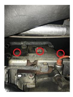
7. The heat shield on the down pipe must also be removed. This is held in place with (3) 10mm bolts.
