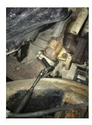
28. Remove the plastic elbow from the factory cold side tube. The end that you will need is labeled CAC. It is recommended to clean the elbow up with engine degreaser and warm water. Install the supplied 3" boot and clamp on the elbow. Reinstall the metal wire clip on to the elbow and slide it onto the intercooler making sure it locks into place.
