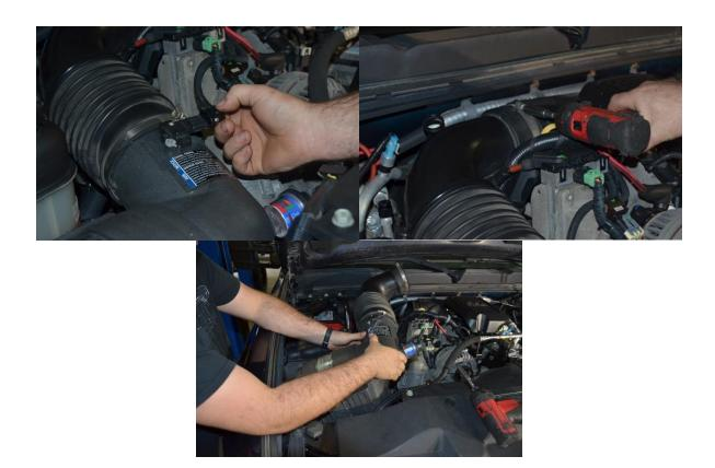
3. Remove resonator box from intake mouth piece. Use a flat head screw driver and loosen the worm gear clamp.
