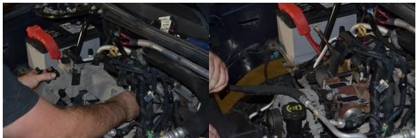
14. Remove the coolant lines from the EGR cooler. If you have not drained the coolant yet you must drain it before removing the coolant lines.
