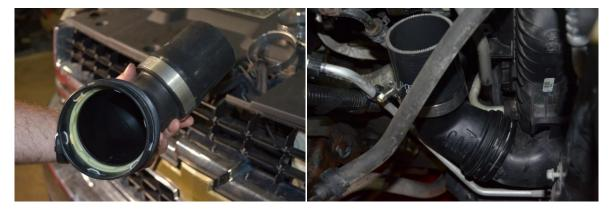
29. Slide the 3" boot and clamp onto the bridge neck. Next install the new cold side placing it into the boot at the intercooler first and then into the bridge neck.
