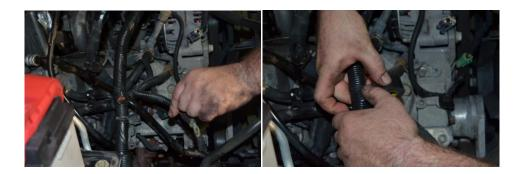
18. Now it is time to remove the bridge neck. There are no bolts holding the neck in, with a rocking twisting motion remove the neck from the bridge. Be careful not to damage the fuel pressure regulator.
