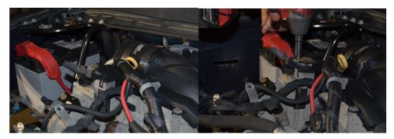
6. Remove the 10mm nut holding the power wire on the alternator.
