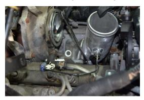
27. Reinstall the steel fuel lines and reconnect them to the rubber lines. Make sure to reinstall the hose clamps.
