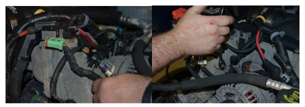
5. Open the cover on top of the grid heater and remove the 10mm nut securing the power wire.
