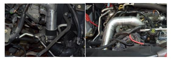
30. Install the MAP sensor in the new cold side using the original bracket and hardware.
