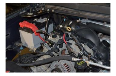
7. Using plyers release the clamp holding the PCV hose assembly to the turbo mouthpiece. Loosen the V-band worm gear clamp holding he mouthpiece to the turbo and remove.
