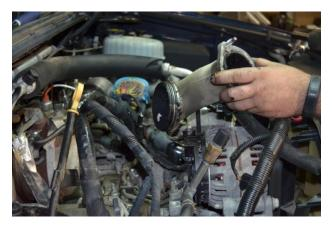
19. It is best to remove the fuel lines that route over top of the bridge. This can be done by removing the nut and stud on the passenger side intake runner, and also the 12mm bolt located just behind the fuel pressure test port. Also don't forget to disconnect the rubber fuel lines from the steel lines.
