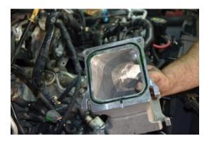
24. Put the new bridge in place the same way the old one came out. With the new bridge in place first install the lower 4 nuts and begin to tighten them in an X pattern. While tightening look at the top 4 holes once the top holes are lined up install the bolts finger tight then continue tightening in a X pattern to 89inlbs both top and bottom.
