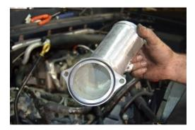
26. Remove the IAT sensor from the top of the old bridge and clean any soot build up off the sensor. With the sensor clean install it into the new bridge neck and tighten.
