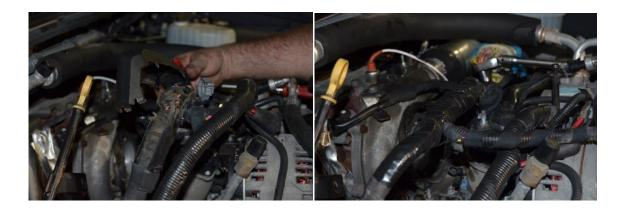
17. There is also a power wire that needs to be eliminated that went to the grid heater. Cut the end of the cable off and wrap the end of the wire with electrical tape or heat shrink and tuck it into the harness and tape it closed.
