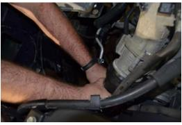
13. Now remove the (6) 12mm nuts and bolts holing the cold side to EGR valve and bridge neck. There is also a 12mm bolt just in front of the throttle valve that will need to be removed. With the bolts removed rock the cold side back and forth with a lifting motion to remove it from the EGR valve.
