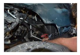
12. Using a pick release the retaining clips from the upper and lower intercooler tube quick connects and remove starting with the intake side first.
