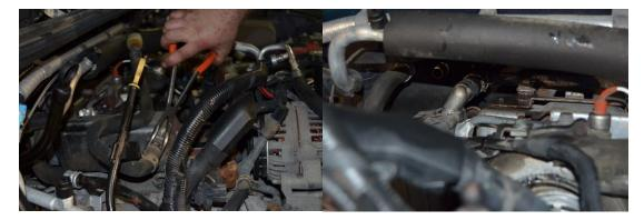
15. Using a 12mm box end wrench remove the two nuts holding the up pipe to the back of the EGR cooler. With the nuts removed now unbolt the (4) 14mm bolts that secure the cooler to the engine. There are two in the front and two in the rear of the cooler. With these bolts removed the cooler will slide out with some careful maneuvering.
