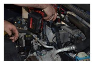
9. Tuck the wiring behind the cold side to get it out of the way.
