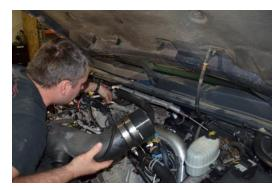
8. Remove the 4 T-30 torques screws holding the plastic wire loom form the top of the cold side.
