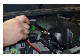
4. Unplug the grid heater, MAP sensor, and throttle valve from the factory cold side. Remove the 10mm bolt securing the harness to the side of the cold side.
