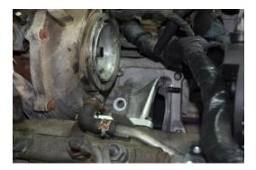
25. Install the new bridge neck on to the bridge using the supplied studs and 12 point 10mm nuts. Make sure the o-ring stays in place. With the nuts installed tighten them with a 10mm boxed end wrench.
