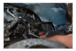
33. Install the intake and filter. Be sure to plug in all electrical connectors. Any connectors not being reused we recommend packing the connectors full of dielectric grease to prevent any corrosion. Fill with coolant and check for any leaks.
